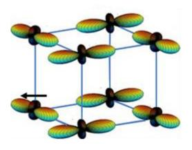
**e.** The spin associated with one  $Mn^{3+}$  cation in LaMnO<sub>3</sub> is shown by the arrow (lower left on the diagram above). Indicate on the picture the directions of the other spins. Is the overall spin ordering in LaMnO<sub>3</sub> ferromagnetic or antiferromagnetic? (2 points)
